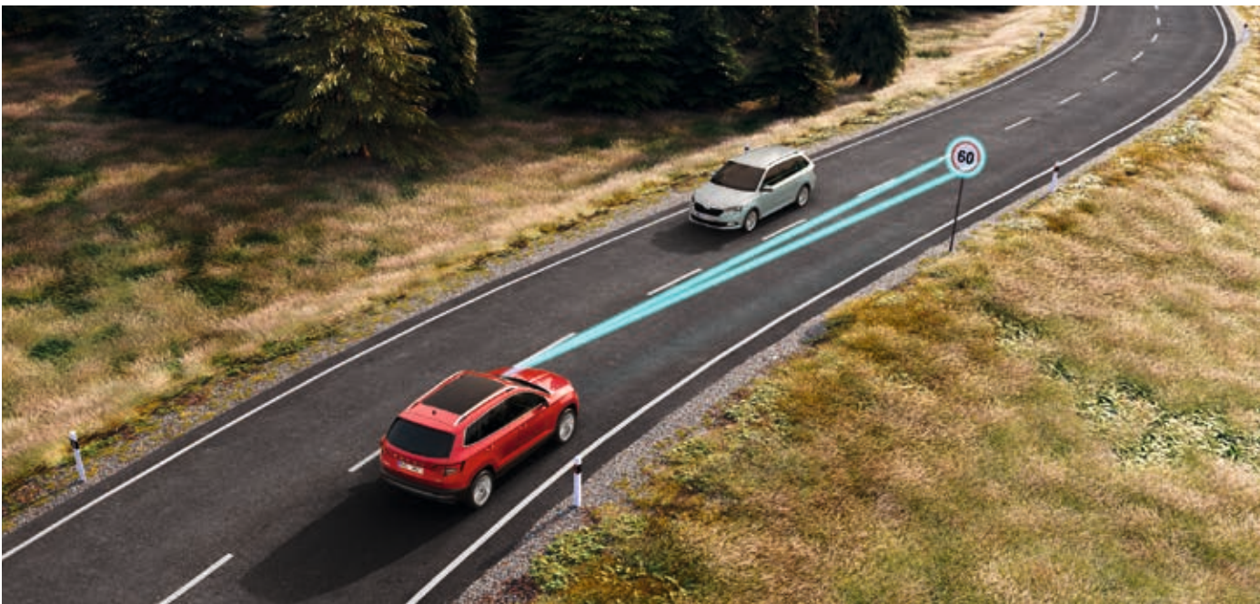
TRAFFIC SIGN RECOGNITION The system uses the camera in the rear-view mirror to scan the traffic signs on the current stretch of road and notify the driver of traffic signs. The system is able to identify signs on both the left and right sides, as well as above the road. Moreover, it is also able to identify variable traffic signs (electronic information boards).
