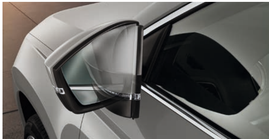
RETRACTABLE MIRRORS The automatically retractable external side-view mirrors fold in when the car is locked, thus protecting them against damage.
