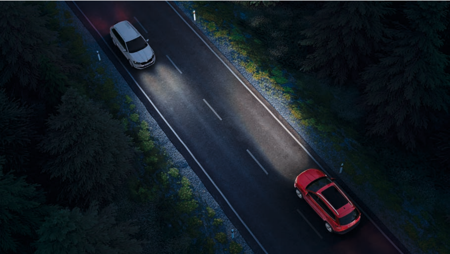
AUTO LIGHT ASSIST Your Light Assist will switch to high beam and back automatically, increasing comfort and safety in traffic.
