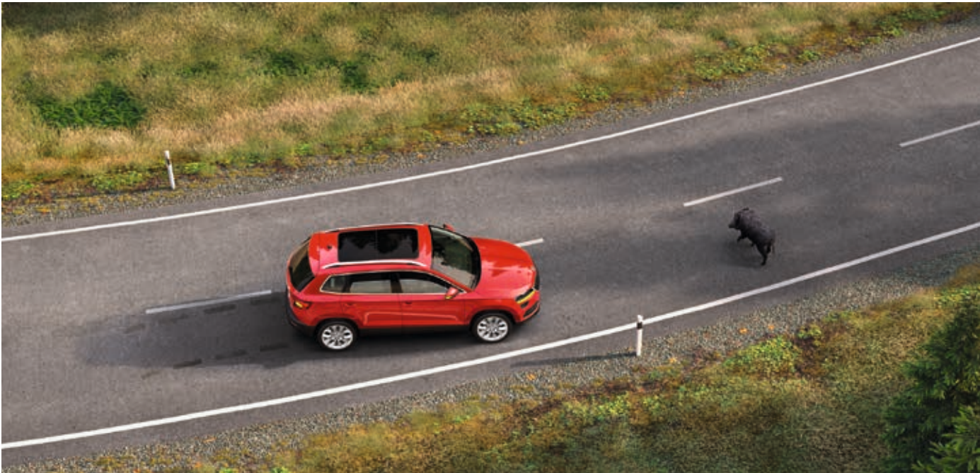
CREW PROTECT ASSIST This assistance system provides increased protection for front-seat passengers in critical situations that could lead to a crash or overturning by closing the side windows to leave only a 5 cm gap, shutting the roof window, and tightening seatbelts.
