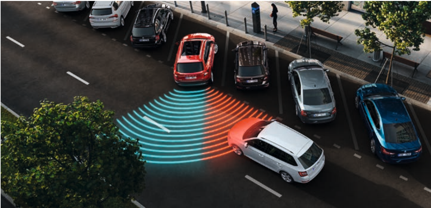
REAR TRAFFIC ALERT The system warns the driver of rear traffic as they pull away from a row of perpendicularly parked vehicles (visually on the infotainment display/ onboard computer display or acoustically), or, if the case so requires, intervenes proactively, i.e., stops the car.
