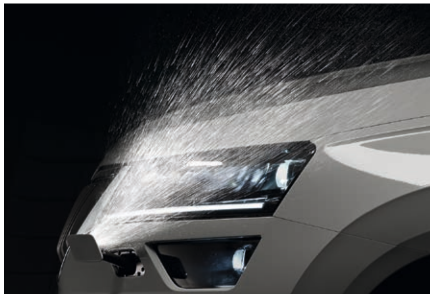
HEADLAMP WASHERS Integrated telescopic headlamp washers easily take care of dust and mud.
